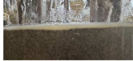
Visible Separation When Low Regolith% Used
