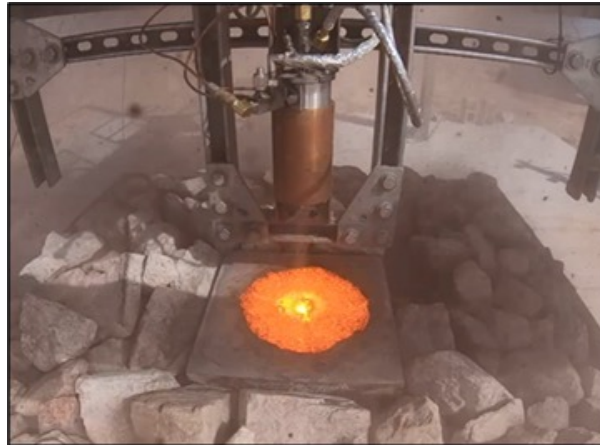
Hot Fire Testing on RENESEST Paver
